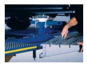
Removable ramp sections lift out easily to give better access to the vehicle.
