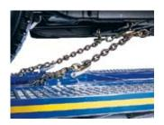
When repairing minor damage, the vehicle can be quickly anchored using B631 chain holders.
