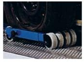
The loading trolley allows you to load immobilized vehicles and can also be used as a vehicle safety stop (just flip it over).
