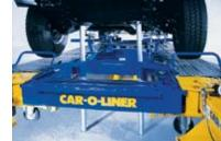
Powerful 10-ton Draw-Aligners pull from almost any angle 360<sup>0</sup> around the vehicle.
