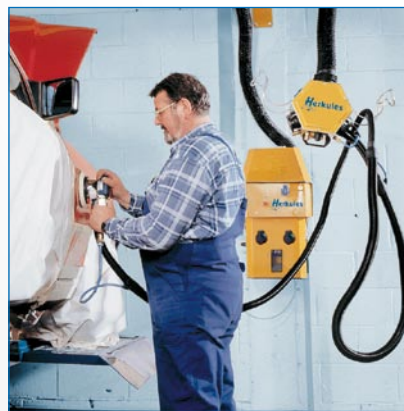
Automatic on / off switching for air- and electrical operated tools.
