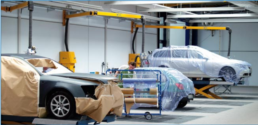
The swivel arms reach to several working places in the preparation area.
