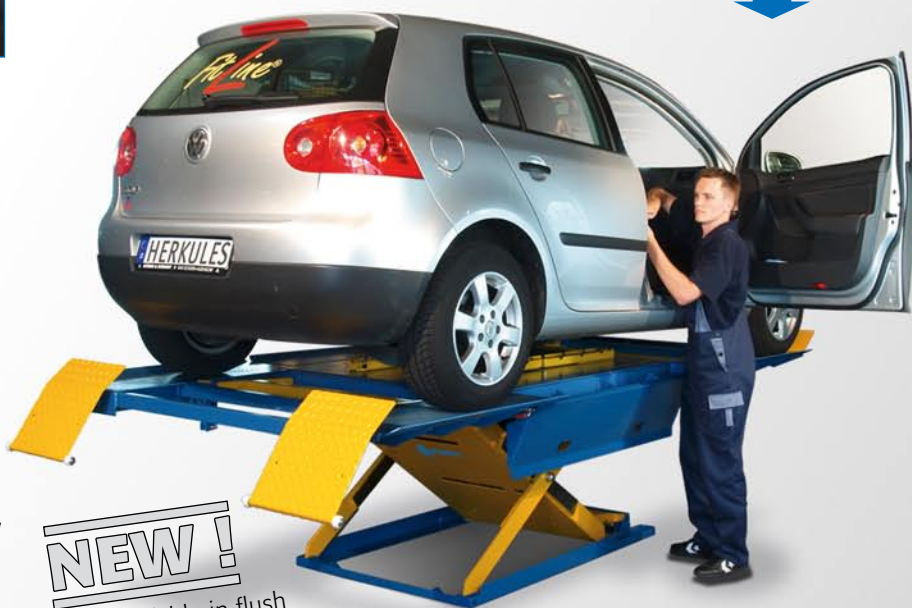
Easy positioning of the liftings points also of extremely flat vehicles.
