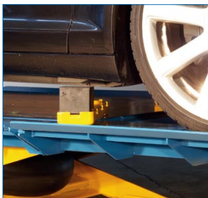
Easy positioning of the liftings points also of extremely flat vehicles.
