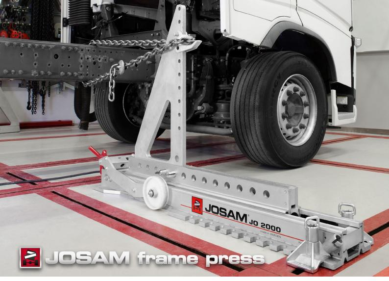
JOSAM frame press with trolley JO 2000, which can both press and pull.
