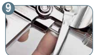
Grease visible part of air piston rod
