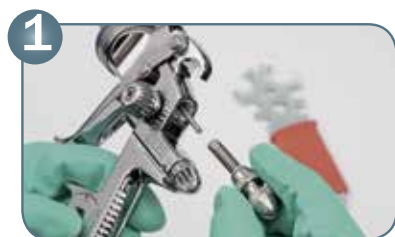
1 First remove paint needle.
