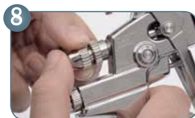
Install material flow control screw
