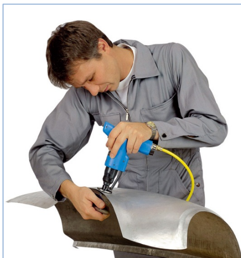
Pilt 102: Pleki venitamine Eckold-pneumovasaraga
